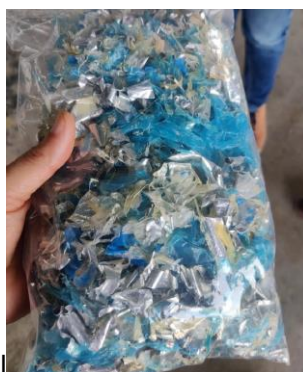
Figure 4: Plastic shredding to be separated into two different fractions (metallised and non mettalised)
